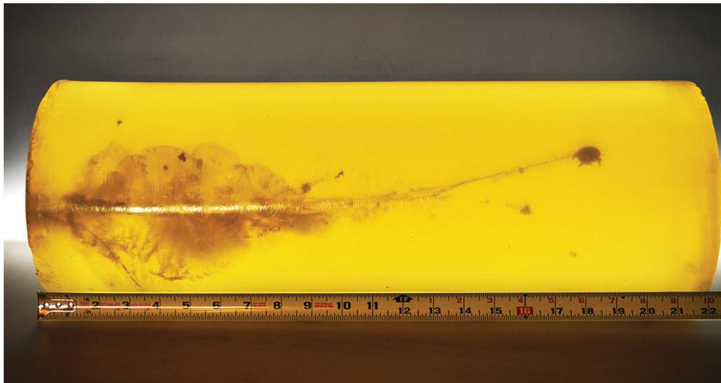
Figure 15. Penetration of a 7.62 Round in a Gelatin Substance.
