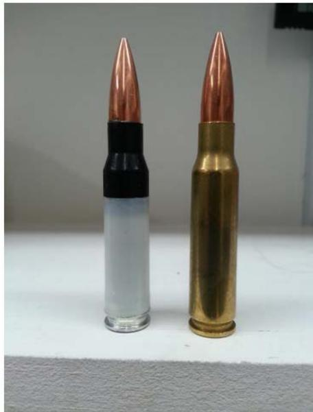
Figure 9. Comparison of Polymer versus Brass Cased Ammunition.
