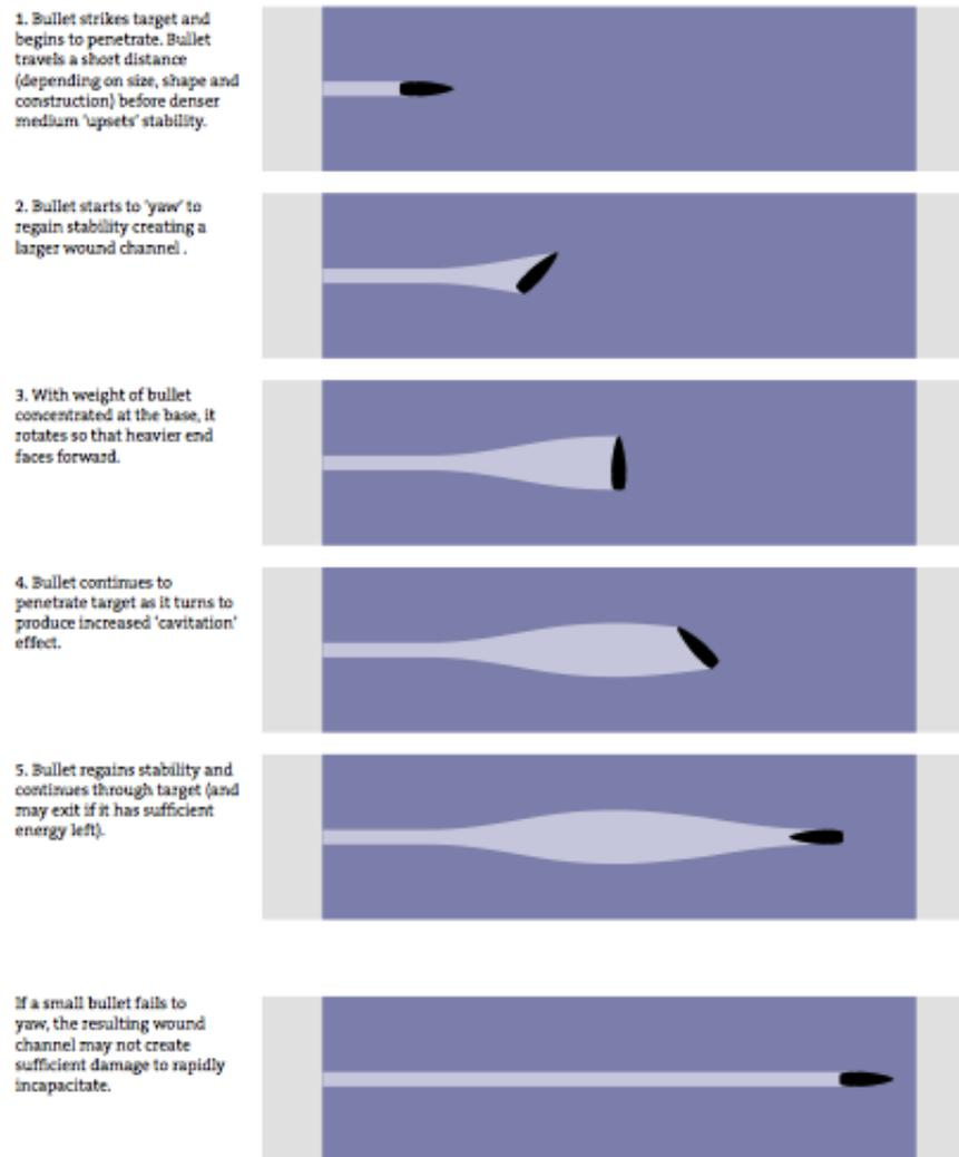
Figure 11. Demonstration of a Yawing Round upon Target Impact.
