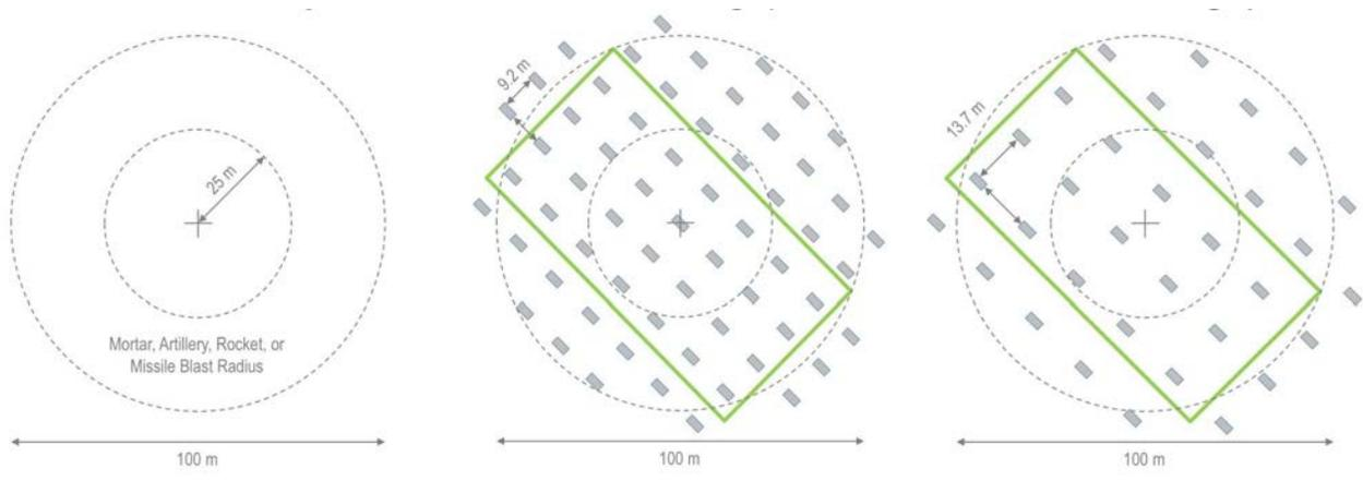
**Vehicle dispersion.** With 30 foot dispersion, 28 HMMWVs fit on a football field. With 45 foot dispersion, 15 HMMWVs fit. **Notes:** Blast effects are not circular. HMMWV is 15 feet long (4.6 m).
