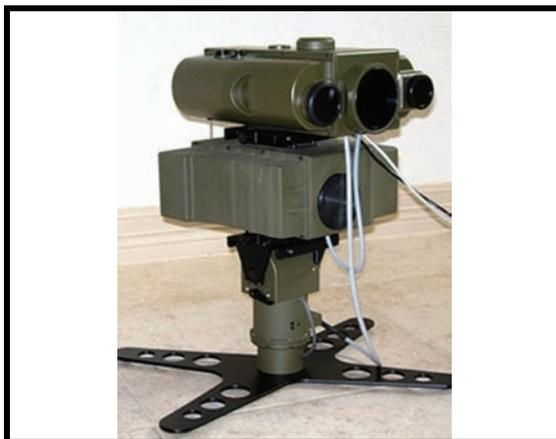
Figure 3-4. Simulated long-range, laser-designator rangefinder.
